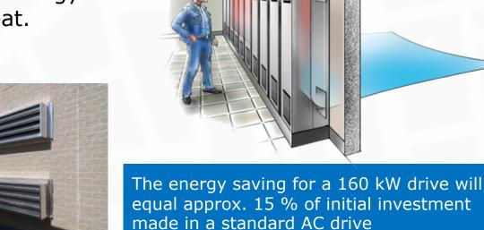
160 kW High Efficient AC drive: Heatloss 2,4%  $\approx$  3.770 W. AC saving ~ 3,77 kW \* 0,9 \* 0,4 AC \* 0,1 US\$ \* 0,6 load \* 24 h \* 365 d = 713 US×/year ~ 15 % of AC drive purchase price per year of operation over the lifetime of the AC Drive
