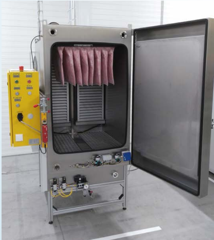
State-of-the-art ISO16890 test duct and discharge chamber in AAF filter lab in Trencin (Slovakia).
