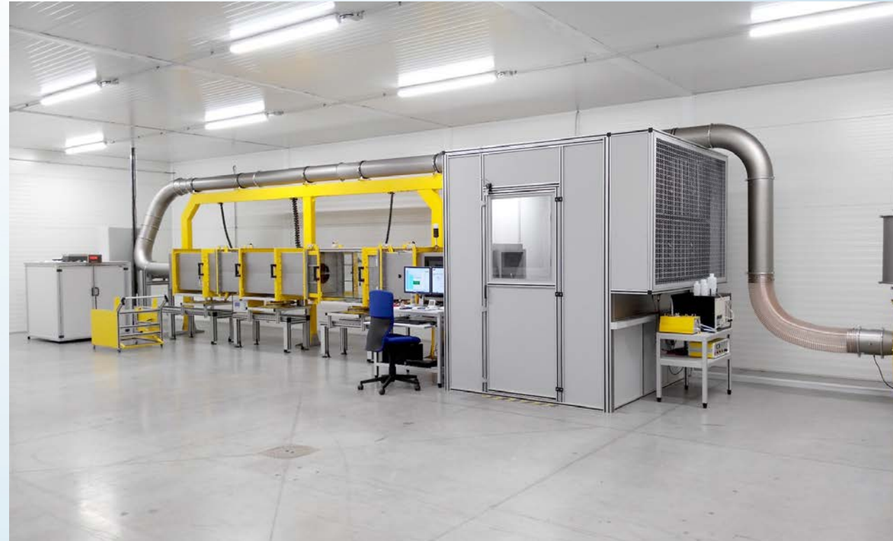
State-of-the-art ISO16890 test duct and discharge chamber in AAF filter lab in Trencin (Slovakia).
