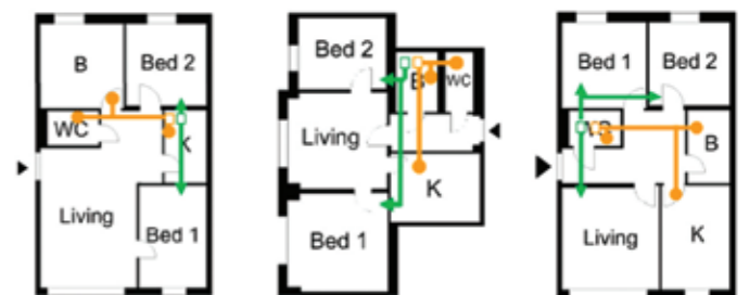
Figure 5: Floorplan examples where extended cascade ventilation (no supply air into living room) is possible (left and centre) and where supply air room into living room is required (right) ©Elisabeth Sibille, University of Innsbruck
