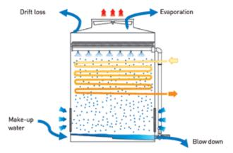
Figure 3: Closed circuit cooling tower
