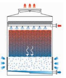
Figure 6: Induced draft, counter flow cooling tower
