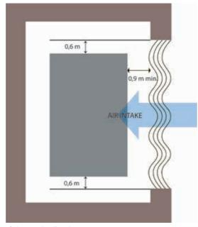
Figure 18: Louvered wall enclosure
