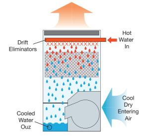
Figure 8: Forced draft cooling tower
