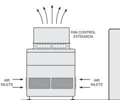
Figure 11: Installation with top of unit at same level of wall
