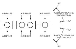
Figure 14: Installation relative to prevailing wind direction
