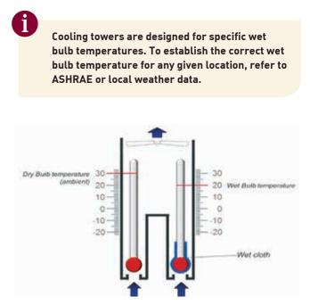
Figure 1: Wet bulb and dry bulb temperatures
