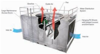
Figure 4: Cross flow cooling tower
