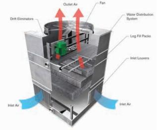
Figure 5: Counter flow cooling tower
