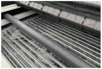
Figure 22: Pressurised spray water distribution
