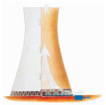
Figure 9: Natural draft cooling tower
