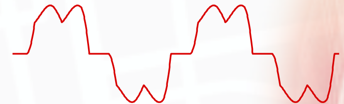
Current distortion caused by non-linear loads in the network
