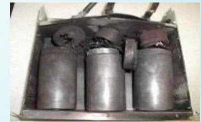
Capacitor Failure
