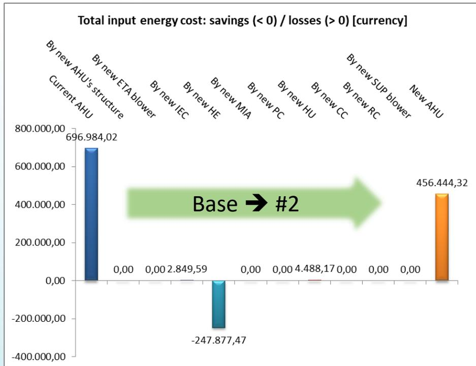
HE's savings @ 100% ODA & CAV (#2) is replaced by bigger savings when modulating ODA @ CAV (#3), both being surpassed by VAV's savings @ modul. ODA (#4): **modulation of both SUP and ODA % gives the best result because it adapts the AHU to the need.**
