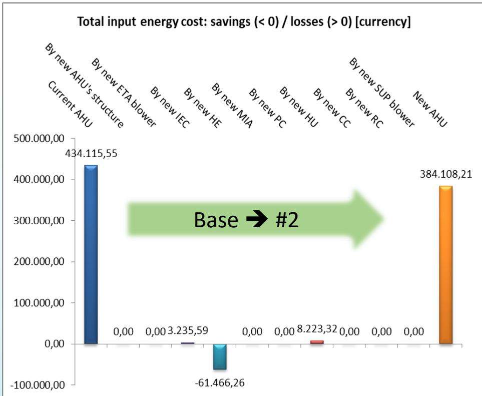
HE's savings @ 100% ODA & CAV (#2) is replaced by bigger savings when modulating ODA @ CAV (#3), both being surpassed by VAV's savings @ modul. ODA (#4): modulation of both SUP and ODA % gives the best result because it adapts the AHU to the need.
