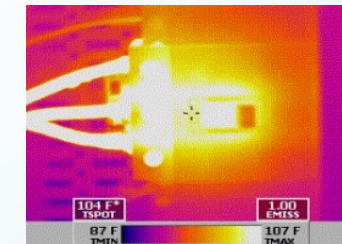
Cable/Contact heating
