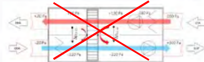
Both fans on building side
